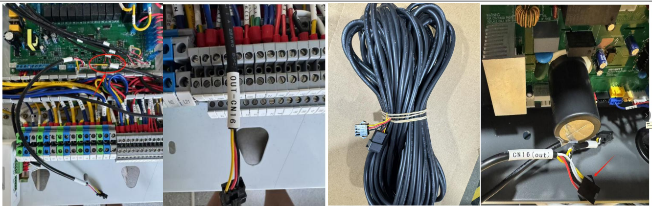
Communication between outdoor unit and another outdoor unit (By 3pin wires)
