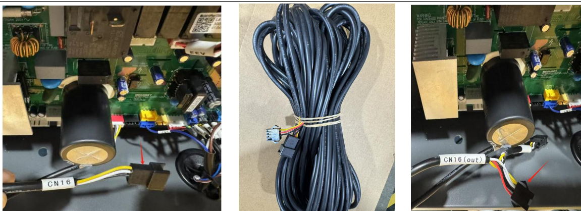
Communication between outdoor unit and another outdoor unit (By 3pin wires)
